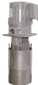
Mechanical seal, multistage close coupled type, for coolant tank cleaning SKM
