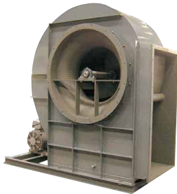
Single inlet belt driven straddle mounted impeller type
